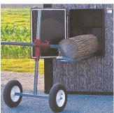
Log Handler is designed to feed big log chunks into a wood stove.
