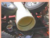
Four pairs of hydraulic-powered tires grab pipe sections, which roll on top of idler wheels. Each driven tire is operated by a separate hydraulic motor.
