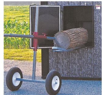
Log Handler is designed to feed big log chunks into a wood stove.
