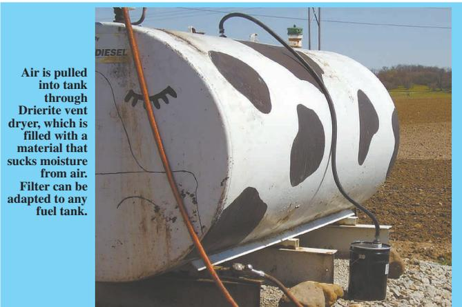
Air is pulled into tank through Drierite vent dryer, which is filled with a material that sucks moisture from air. Filter can be adapted to any fuel tank.
