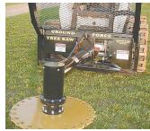
Saw has a rotating feature, which allows the head to rotate from a horizontal to vertical position for delimbing trees.
