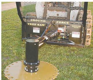
Saw has a rotating feature, which allows the head to rotate from a horizontal to vertical position for delimiting trees.
