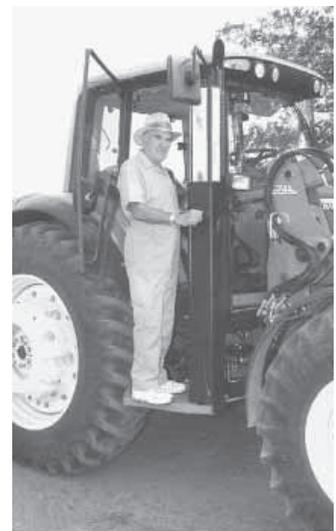
To get into the cab, the operator stands on the lift, opens the tractor door, reaches inside and presses a switch. The lift raises him to the cab.
