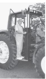
To get into the cab, the operator stands on the lift, opens the tractor door, reaches inside and presses a switch. The lift raises him to the cab.
