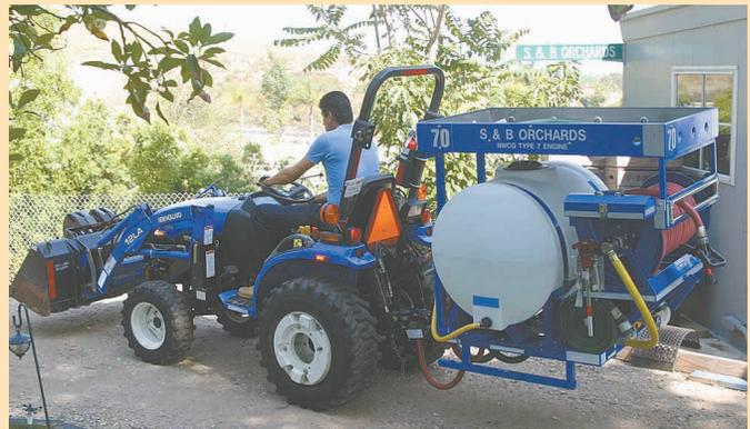
George Edwardz had a modified 3-pt. sprayer custom built and attached a pump and a 110-gal. water tank.
