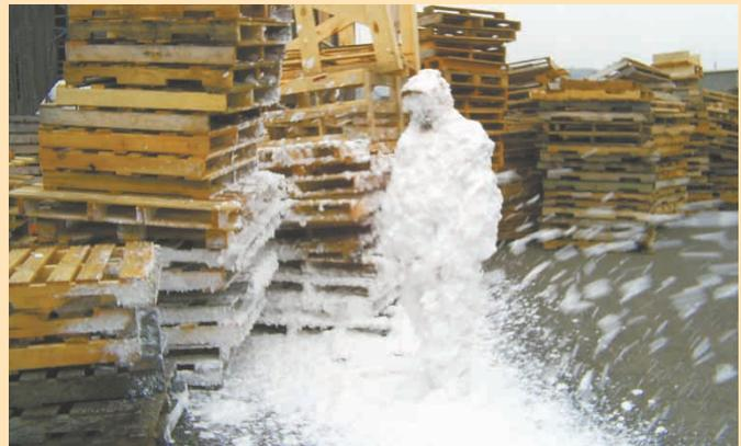
Foam sprays out 50 ft. or more. Each gallon of water produces 20 gal. of foam.
