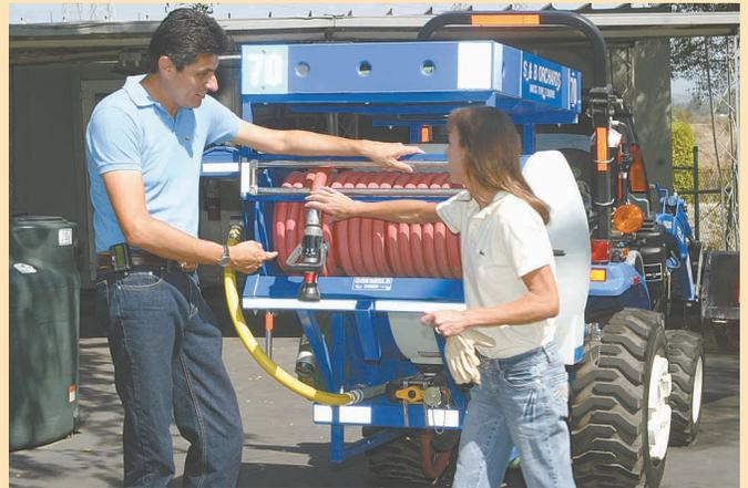
He purchased a \$250 nozzle and 300 ft. of fire hose. The 1-in. fire hose can shoot a 100-ft. stream of water at 30 gpm.
