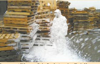
Foam sprays out 50 ft. or more. Each gallon of water produces 20 gal. of foam.
