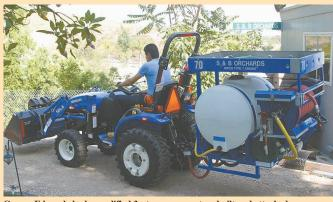
George Edwardz had a modified 3-pt. sprayer custom built and attached a pump and a 110-gal. water tank.
