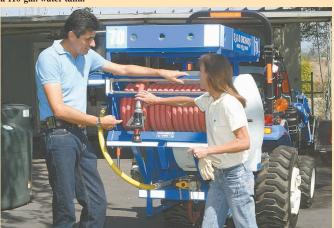
He purchased a \$250 nozzle and 300 ft. of fire hose. The 1-in. fire hose can shoot a 100-ft. stream of water at 30 gpm.
