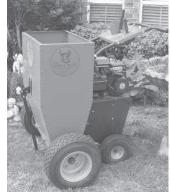
Compost spreader has a built-in agitator that shifts material back and forth to avoid clogging up the holes.
