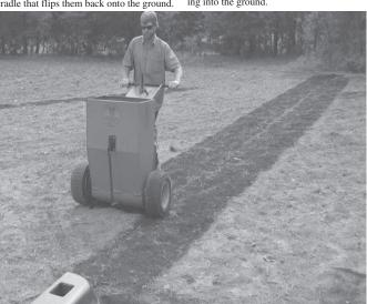
Unit spreads compost anywhere from 1/4 in. to 3 in. deep over a 2-ft. width.
