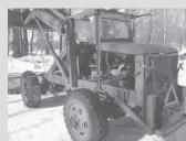
Tractor is powered by a 1969 Chevy 350 with a 400 Turbo automatic transmission. It has three speeds forward, one reverse.
