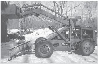
Povlis's loader tractor uses a 6-WD Army truck frame and running gear as the base.
