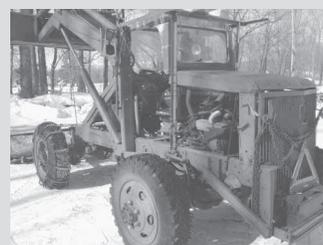
Tractor is powered by a 1969 Chevy 350 with a 400 Turbo automatic transmission. It has three speeds forward, one reverse.
