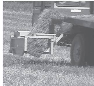
Attachment fits onto side of New Holland stacker. As bales are picked up, they move across machine into a cradle that flips them back onto the ground.
