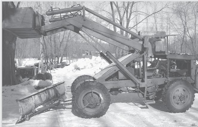
Povlis's loader tractor uses a 6-WD Army truck frame and running gear as the base.
