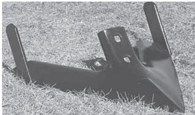
**Twin fins measure 4 1/2 in. high and are welded to the sweep at an angle. They keep tap-rooted weeds from slipping around outer edge of shovel blades, cutting them off.**
