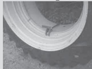
**Steel tool is equipped with a handle that acts against a long rod. Pushing down on handle provides the leverage to extend the rod and push wheel off.**
