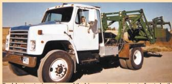
Truck has two steering systems, and the driver uses two separate sets of controls - the original ones for highway use, and another set of controls for operating the loader.
