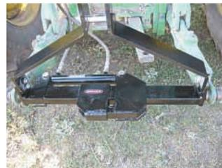
Hitch can be easily transferred to another tractor since it just pins in place on drawbar.
