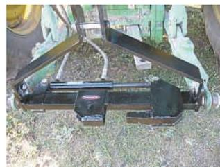
"Quick Hitch" uses a hydraulic ram to slide a hitch mechanism back and forth on drawbar, "grabbing" the pin on a wagon or implement.
