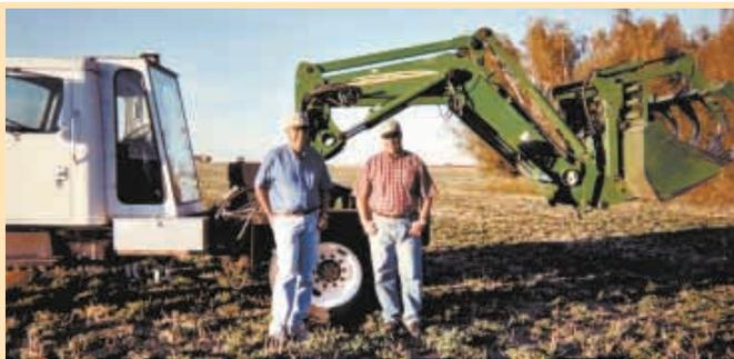
Rein Grinding converted a used 1980 IH 2-ton truck into a "reversed" heavy-duty loader tractor. They use the rig every day to custom grind hay for local feedlots.
