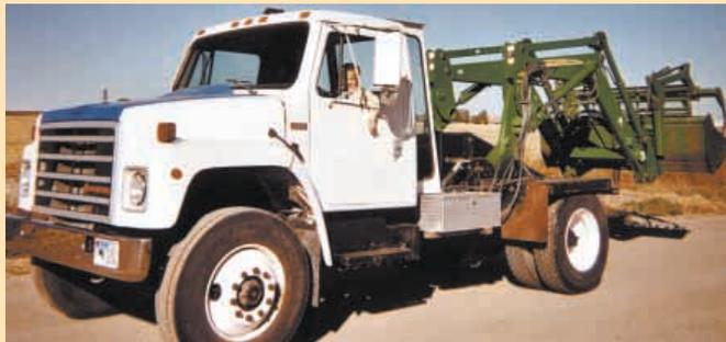
Truck has two steering systems, and the driver uses two separate sets of controls - the original ones for highway use, and another set of controls for operating the loader.
