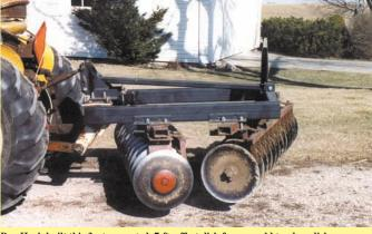
Ben Hach built this 3-pt. mounted, 7-ft. offset disk from an old tandem disk.
