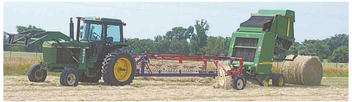
Cecil Scott modified an H&S 27-ft. rake to pull his round baler. "It eliminates the need for a separate raking pass and turns baling hay into a one-man operation," he says.
