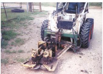
Skid loader-mounted tree "slicer" uses a cutterhead off a New Holland pull-type silage harvester. "It'll cut trees up to two inches in diameter," says Charles Hardenburger.
