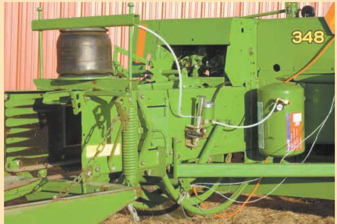
Airbaler kit replaces manual and hydraulic tensioning rods above bale chamber. Airbag mounts directly above bale chamber, fed by air from a small tank (at right in photo).
