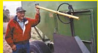
to raise and lower the wagon's slide gate. If the wheel still turns hard, an 18-in. long extender pipe can be added.
