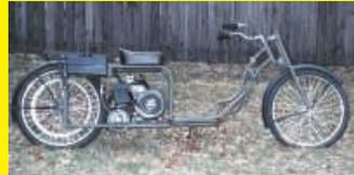
bike. It runs and handles real nice. The frame is made out of 1-in. sq. tubing and 1-in. water pipe with 24-in. spoke bike wheels. I made the front fork with knee action and part of an old front end off a girl's bike. The seat came from an old scooter. **(Hiram Wilson, 315 Bonnaridge Dr., Hermitage, Tenn. 37076 ph 615 883-1177).**
