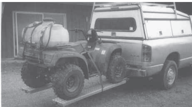
Lester Langeland made an ATV carrier that mounts on back of a pickup, allowing him to transport an ATV even with a topper on the pickup bed.
