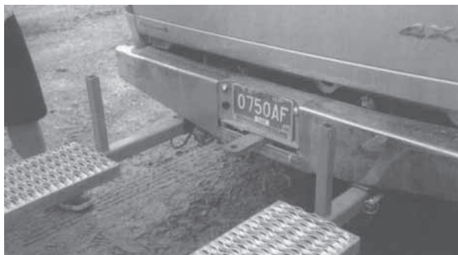
Ramps slide into a pair of metal brackets that mount permanently on pickup frame.
