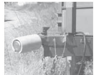
“DaPlug” trailer lock (left) is designed for lunette ring or pintle hitch trailers. “DaBull” (right) is designed for Bulldog-type hitches. Both fully encase the hitch to protect the lock.
