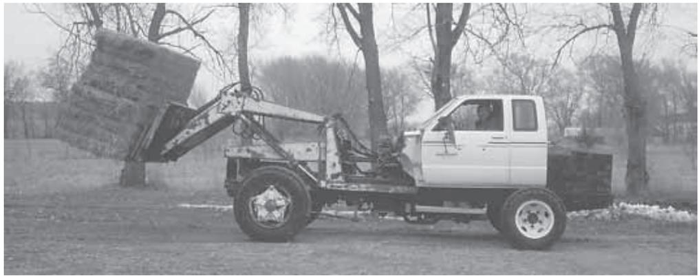
Heads turn whenever Vern Schneider goes to pick up big square bales. He bolted a mid-1980's S-10 pickup cab onto a 1975 2 1/2-ton Chevy truck frame and attached a used loader on front. Forklift weight box on the rear helps balance the weight of the bales.
