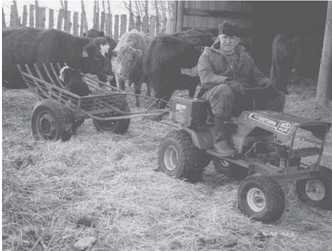
Electric-powered "ATV" is really a converted Sears Craftsman riding mower.
