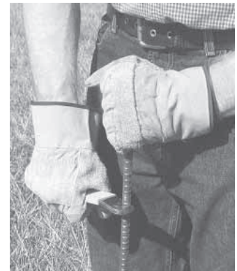
To remove a post, you slip notch over post and pull up on tool while grabbing top of post with your other hand to keep it steady.
