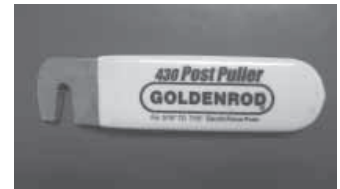
Goldenrod post puller has a deep, tapered notch at one end with small gripping "teeth" embedded in it.
