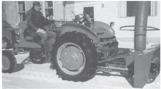
Lyle Rawn mounted an extra seat, steering wheel, and controls on one side of his AC tractor, allowing him to operate it in reverse with the snowblower in front of him.
