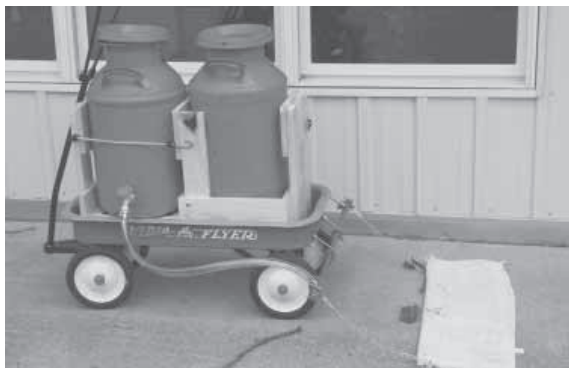
Hand-pulled Zamboni is made out of two milk cans, a Red Rider wagon, and hoses. It lays down a thin layer of hot water, just like a real Zamboni.
