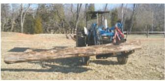
"It lets me pick up a log and turn it into firewood lengths in no time at all," says Fred Miller about his home-built log clamp. Mounts on either a skid steer or a tractor loader.
