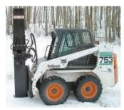
"Post-Vibe" fence post driver quick-taches to skid steer loaders or farm tractors. It vibrates posts into the ground.
