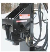
A cup on bottom of vibrator holds top of post so it can't move or deflect sideways.
