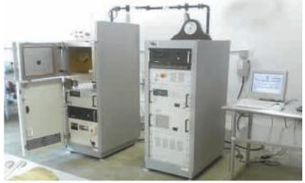
Original GRC "fuel maker" uses microwave emitters to make fuel out of everything from tires and oil shale to biomass and plastics.
