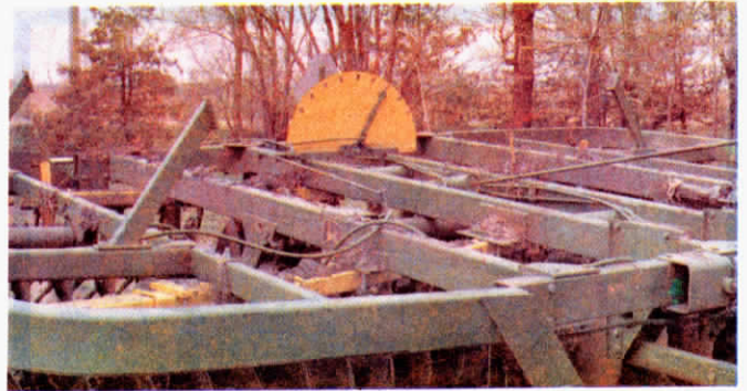
All you do is tell driver which number of the dial marks the depth you want the disk to run.
