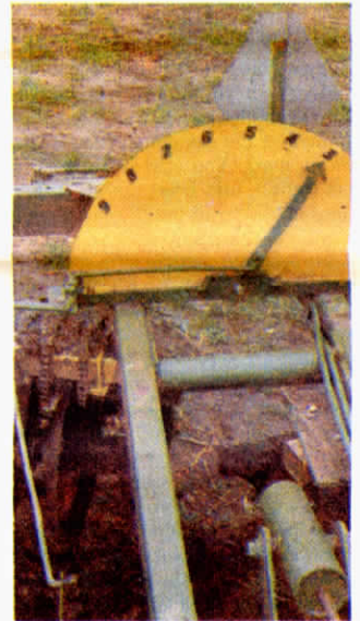
Close-up photo shows how home-built dial is hooked up to constantly monitor depth.
