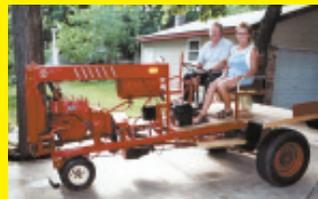
housing from an industrial asphalt trailer. A friend gave me a 3/4-ton rear end and 4-speed transmission out of a 1973 Ford pickup, so I made a steel frame and went to work. The clutch is dual belt-driven and the starter is also belt-driven by a 12-volt motor. The machine has rear hydraulic brakes.
