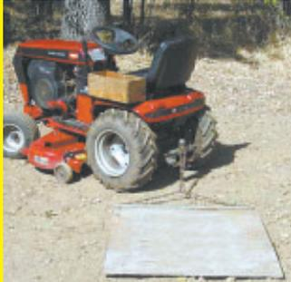
A simple "stone boat" is an easy way to haul large rocks and other heavy loads around the farm. Just run a chain back to a piece of plate steel and tow it behind a garden tractor. It tows easily and you don't have to do any lifting. You can just roll loads onto it. **(Maurice Leighton, Citrus Heights, Calif.)**
