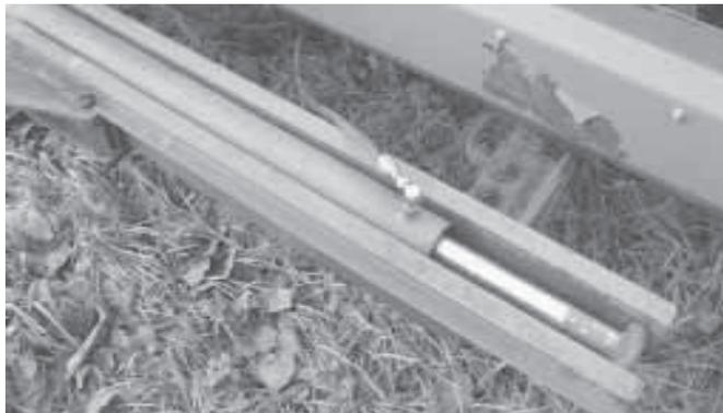
Hydraulic hitch is made of 4-in. sq. tubing bolted onto original transport hitch and harvester's blower housing. Hydraulic cylinder can move up to 30 in. back and forth.
