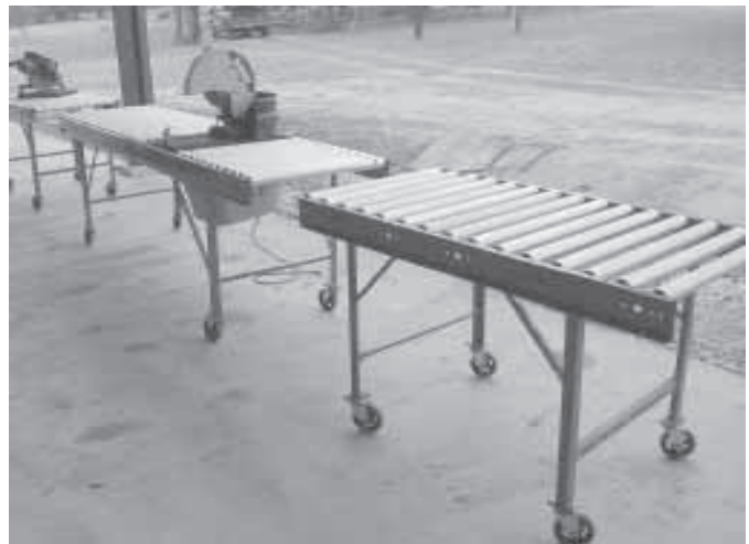
Saw sits in middle of one 10-ft. roller section. The other roller section was cut in half to provide two 5-ft. sections.
