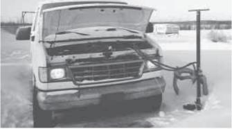
A 12-volt pump plugs into van's battery and is used to pump anti-freeze through hoses from the ground into the engine.
