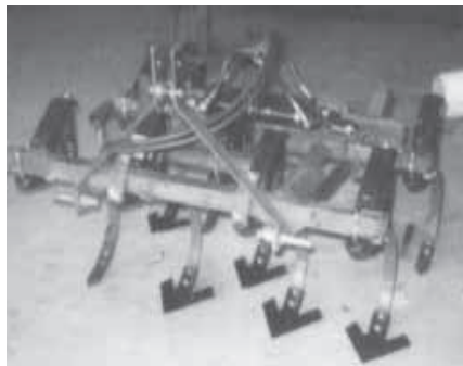
Cultivator is made out of 2 3/4-in. sq. tubing that goes into 3-in. sq. tubing receivers to expand and decrease width of cultivator hydraulically.
