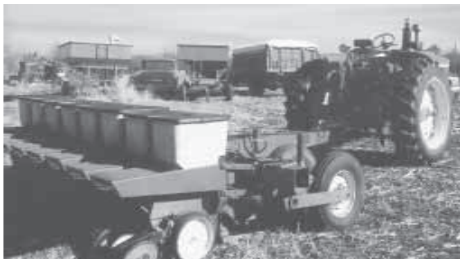
Edgar Phillips uses this 8-row, 15-in. Deere 7000 planter which was converted from an 8-row, 30-in. model.
