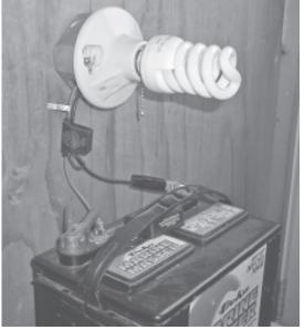
The 12-volt fluorescent bulbs can be hooked up to batteries.
