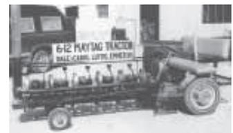
Luttig built a tractor powered by Maytags. The motors are timed to run at the same speed.
