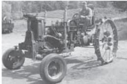
"I'm impressed at how well it runs," says Bill Harris, who repowered a 1934 Farmall F-12 tractor with a Subaru car's fuelinjected engine.
