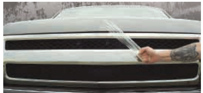
Pre-cut clear plastic film covers the areas of your car or truck that are most likely to be damaged by rocks, bugs and scratches.
