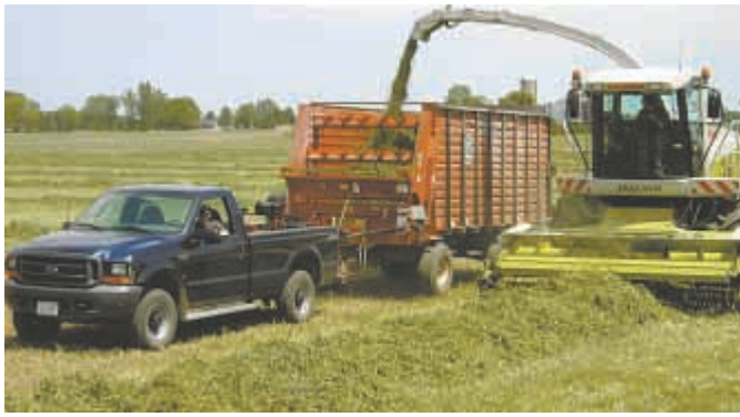
Hydraulic pto power unit lets you use your pickup to operate rear unload forage boxes.
