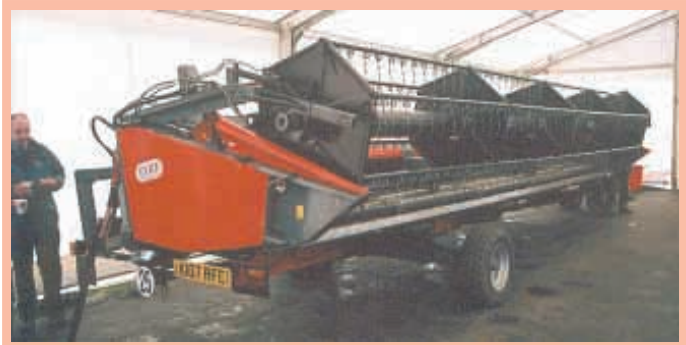
Crop material from 25-ft. swath feeds evenly into a 25-ft. wide threshing drum, which avoids bottlenecks and requires a lot less power while boosting productivity.
