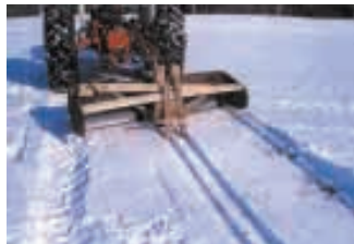
When downpressure is applied to blade, the skis leave deep parallel tracks to follow while cross country skiing.
