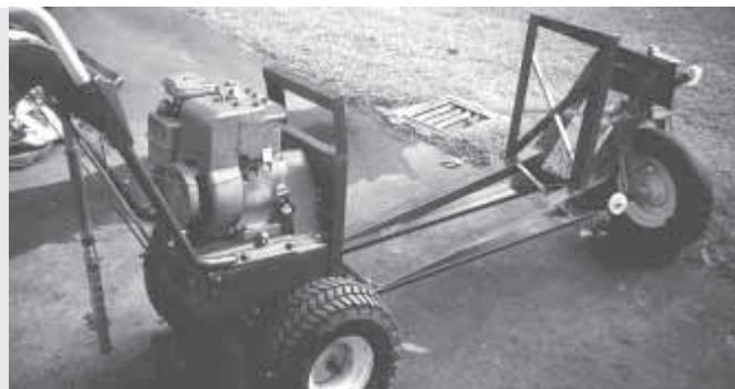
**Arthur Moulton built this self-propelled wheelbarrow out of an old Ariens snowblower and junk parts. It's shown with the wheelbarrow bucket removed.**
