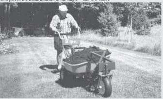
Dump-style, sideways-mounted bucket can be bolted to wheelbarrow.
