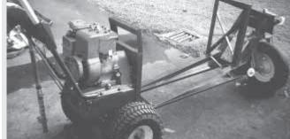
Arthur Moulton built this self-propelled wheelbarrow out of an old Ariens snowblower and junk parts. It's shown with the wheelbarrow bucket removed,
