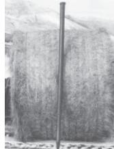
A 7-ft. metal shaft can be used to create pilot holes for wood posts, says Thomas.
