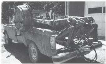
Hydraulic-powered spinning tractor tire rim, activated by flipping a toggle switch, is used to roll up barbed wire.
