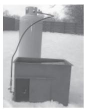
Liquid propane heats water in tank, which is equipped with a burner that sets inside a metal box welded to one corner of tank.
