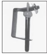
Simple locking bar keeps equipment safely secured to tractor.
