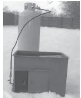
Liquid propane heats water in tank, which is equipped with a burner that sets inside a metal box welded to one corner of tank.
