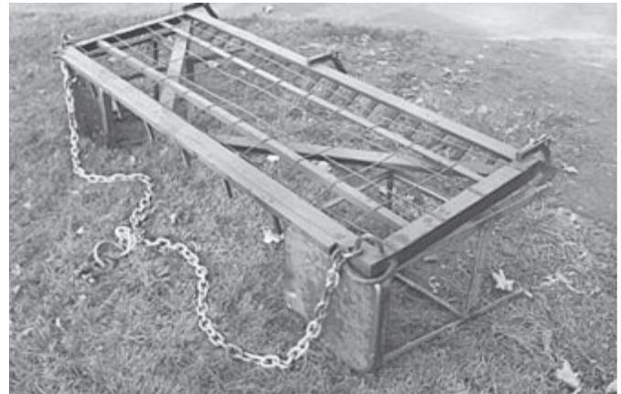
"Track drag" uses 4 1/2-in. long angled steel spikes to loosen the soil.
