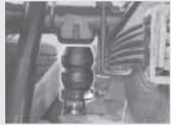
Hollow rubber springs are available for front and rear axles as well as trailer suspensions.
