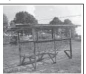
Metal feeder is designed to hold two round bales and has a 10 by 12-ft. roof. "It supplies enough feed for my goats for several weeks at a time," says inventor Wade Hearn.
