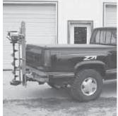
"Auger mount" transports augers and holds it while you dig. It can be used on both  $ATV\sapers$  (left) and pickups.
