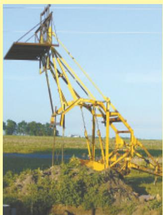
He welded an A-frame structure to baler’s tailgate to support a 4 by 10-ft. treated wood platform with safety rails on each side. It lifts up to 15 ft. off the ground.
