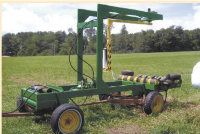
Strawser used the running gear off a light-duty wagon to build his own bale wrapper. The arm that holds wrapping material was bought from a bale wrap manufacturer.
