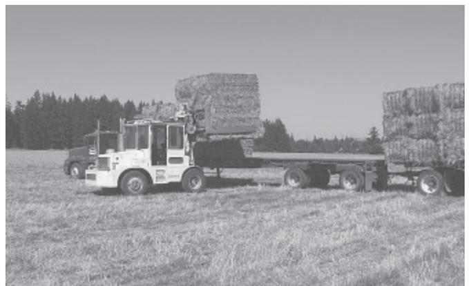
Loader tractor can pick up and stack six 3 by 4-ft. big square bales three high on a semi truck or nine high in a barn.
