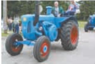
hp Lanz Bulldog would only consume a gallon of diesel fuel per hour. The one-cylinder tractor ran at a top 850 rpm's.
