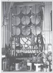
makes it easy to store various fuels and chemicals. The rack is made out of channel iron and square tubing and extends almost as high as the shop's ceiling. It had been built by someone else and I bought it at an auction. I store 50-gal. oil barrels on the rack's shelves, and I use a gear-type pump to fill them and also to drain out the oil as needed."
