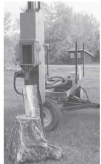
Fence post pounder is fitted with a home-built splitting axe attachment.
