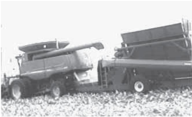
Vernon Flamme's cob collector uses a conveyor to deliver cobs into trailing side dump wagon. System is powered by a diesel engine that direct-drives a hydraulic pump.
