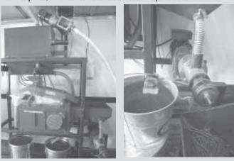
The O' Briens burned more than 2,000 gal. of canola oil in their equipment in 2007. Extruder squeezes oil out of canola and makes "pellets" out of the meal (left).
