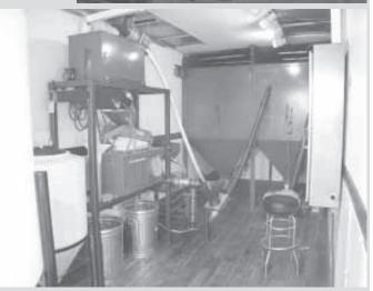
Unit can produce 80 gal. of canola oil every 24 hours and extrudes the leftover canola meal into pellets, which can be fed to cattle or used in a pellet stove.
