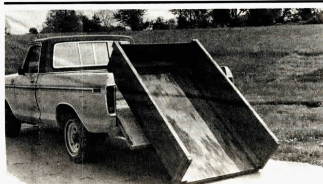
Box dumps by quick stopping in reverse. It then rolls easily by hand back into pickup bed.
