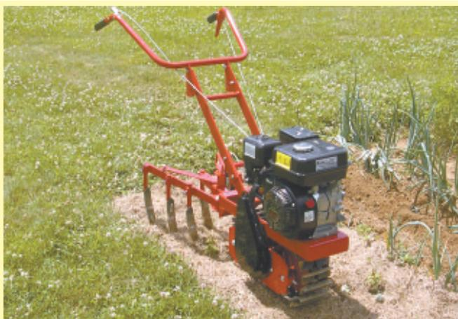
Tracked Ground Hog Cultivator works like a rototiller, pulling rear cultivator tines.
